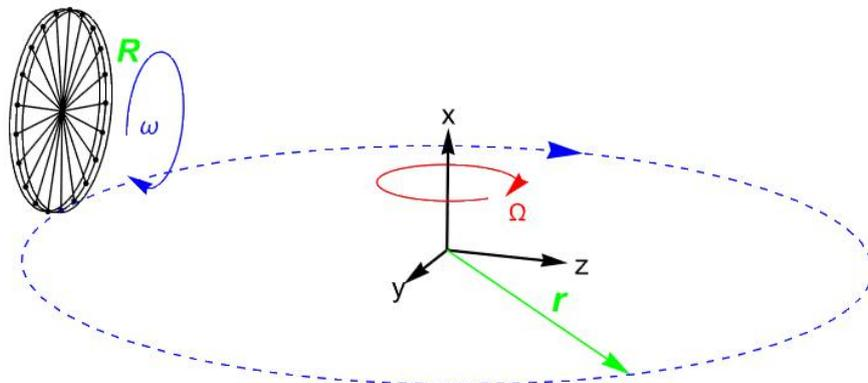
$$\vec{M} = \frac{d\vec{L}}{dt} = \vec{\Omega} \times \vec{L} = \begin{pmatrix} -\Omega \\ 0 \\ 0 \end{pmatrix} \times \begin{pmatrix} \Theta_x & 0 & 0 \\ 0 & \Theta_y & 0 \\ 0 & 0 & \Theta_z \end{pmatrix} \begin{pmatrix} -\Omega \\ 0 \\ -\omega \end{pmatrix} = \begin{pmatrix} 0 \\ -\Theta_z \cdot \omega \cdot \Omega \\ 0 \end{pmatrix} = \begin{pmatrix} 0 \\ -\Theta_z \cdot \Omega^2 \cdot \frac{r}{R} \\ 0 \end{pmatrix}$$
