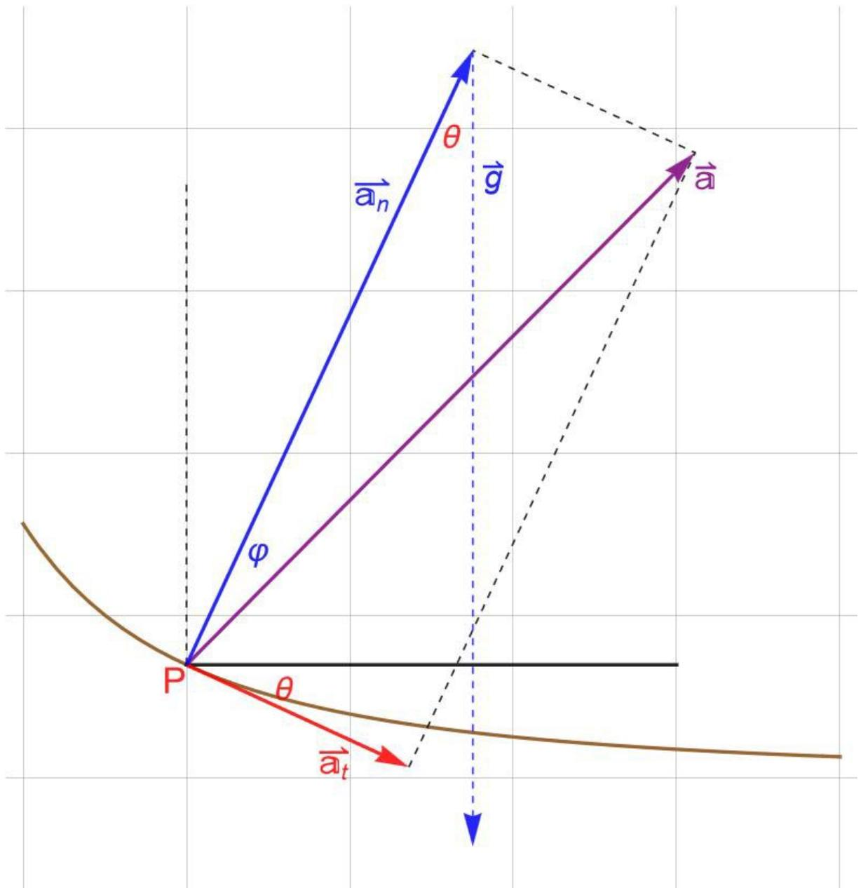
$$a_n = \frac{v^2}{\rho} = \frac{\left(\frac{125 \text{ m}}{18 \text{ s}}\right)^2}{5,78 \cdot \text{m}} \approx 8,34 \frac{\text{m}}{\text{s}^2}; a_t = 3 \frac{\text{m}}{\text{s}^2};$$
