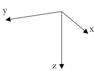
$$\frac{d\vec{e}_\omega}{dt} = \vec{e}_y = \overbrace{\dot{\varphi} \cdot \vec{e}_z \times \vec{e}_y}^{\vec{v} = \vec{\omega} \times \vec{r}} = \overbrace{\dot{\varphi} \cdot \vec{e}_{-x}}^{\vec{e}_z \perp \vec{e}_y} = \Omega \cdot \vec{e}_{-x}$$
