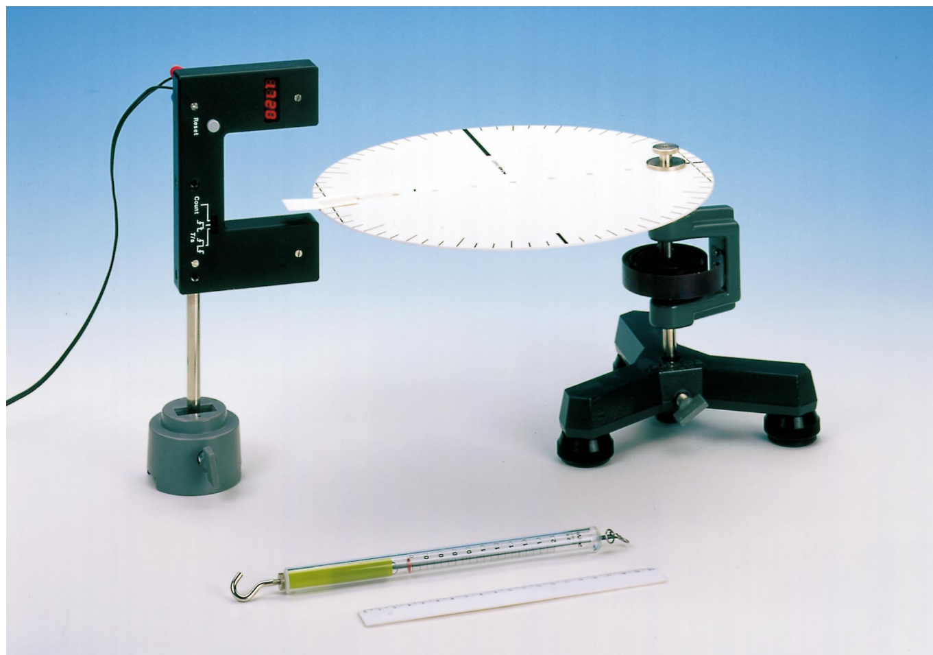
Fig. 1: Experimental set-up for measuring the moment of inertia (Steiner's theorem).
